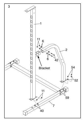
4. Slide the remaining Brace (2) onto the bracket on the other Upright (1). Attach the Brace to the Upright with two M10 x 65mm Bolts (42), four M10 Washers (6), and two M10 Nylon Locknuts (11). Do not tighten the Nylon Locknuts yet.
